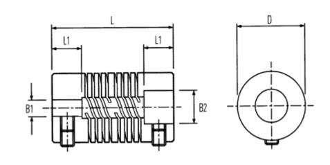
B1: Pre-drilled= 4.8B2: Pre-drilled= 6.35D= 19.1L= 26.5L1= 6.5Max angular displacement = 0.25Max B1 & B2= 10.00Max parallel displacement = 7
